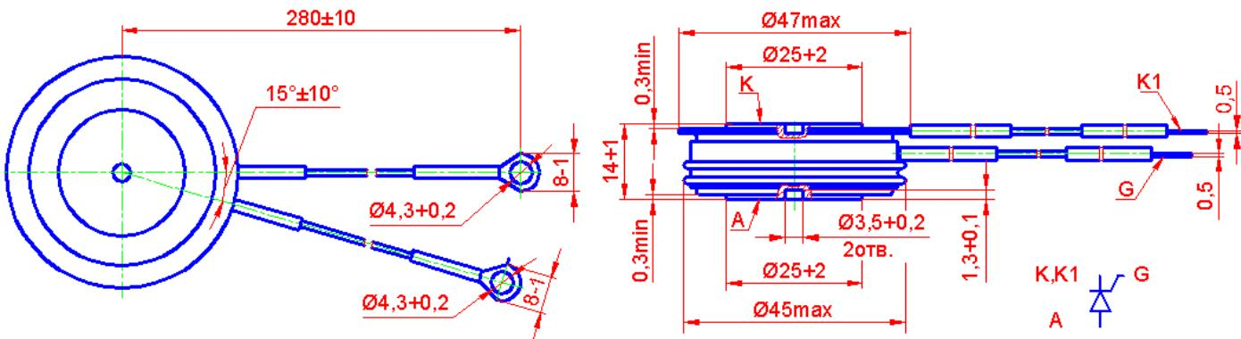
Tightening torque : 9 ÷ 12 kN
